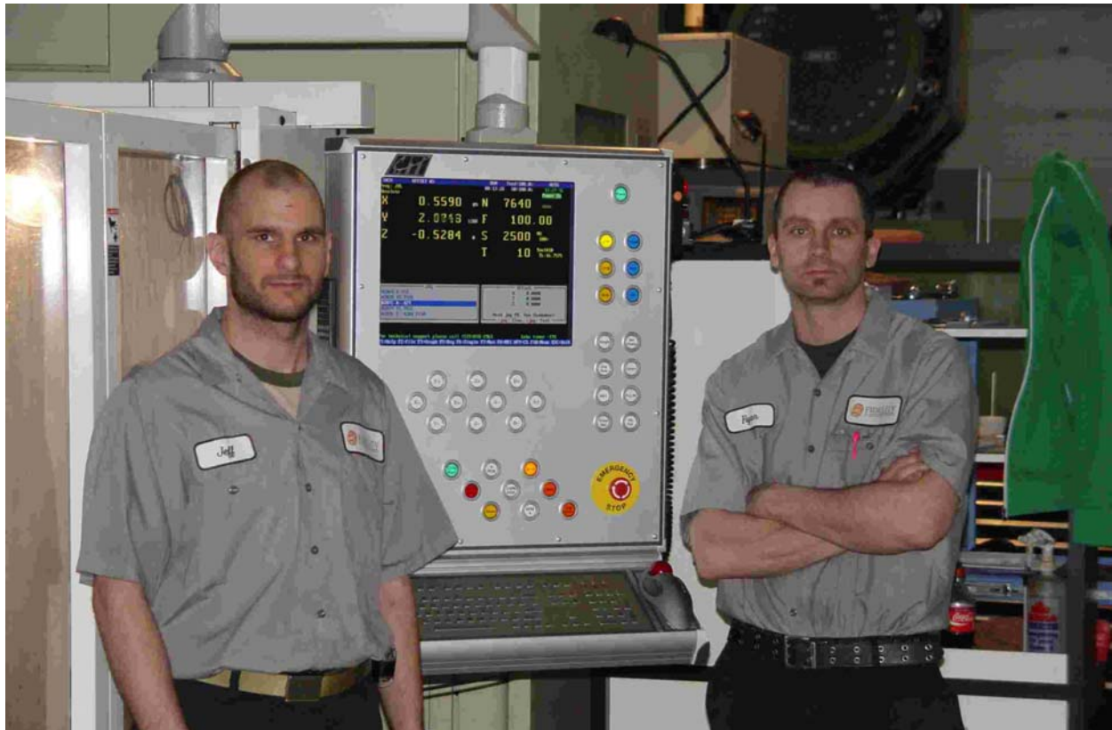
Jeff Litster (left), co-owner of Fidelity Machine and business partner Ryan Arsenau in front of their 1997 Fadal machining center with its MTI Constant Velocity Controller. “With older controllers you really can’t trust the finished product,” said Litster, “which leads to slower cutting, more checking and more scrap.”
