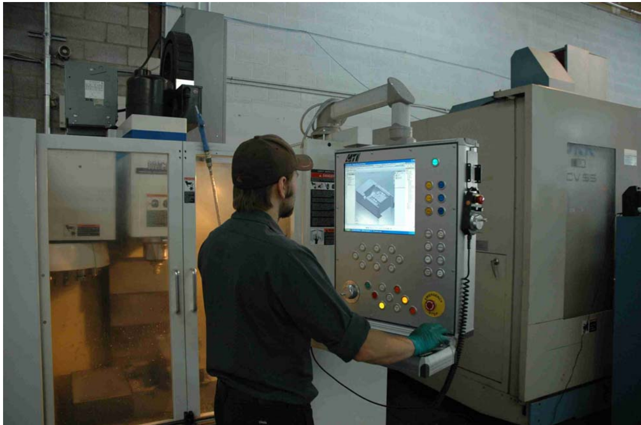
Machinist Joe Brunelle at work at Fidelity Machine & Mould cutting a cable-over-mold job on their 1997 Fadal VMC15 retrofitted with the MTI Constant Velocity Controller.
