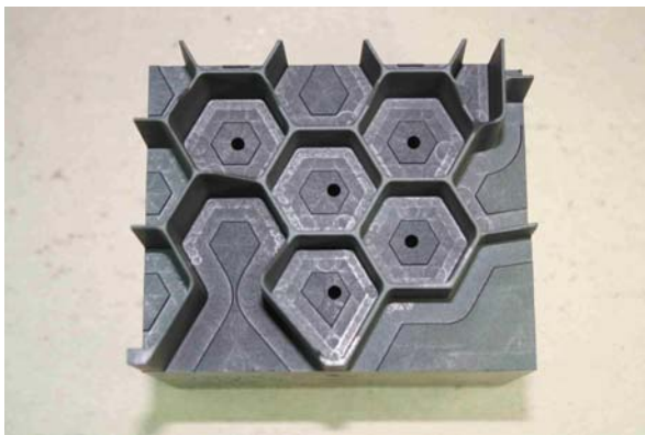
Above, two more close-up views of another graphite electrode for a console component. Below left, a CAD rendering of that tool. In the rendering, green areas represent the molding surface or area to be burned. Light blue areas indicate clearances to avoid interfere with other areas in the tool. This job is for an automotive customer.
